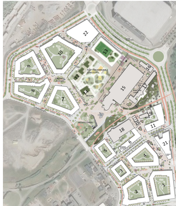
Figure 3. Site plan of Flytårnet neighborhood, from [5]. Buildings marked in gray (15–16–17–18–19) are existing buildings planned for renovation, while those in white will be newly constructed.
