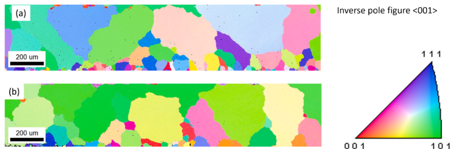
Fig. 12. EBSD inverse pole figure (IPF) maps (superimposed with grain boundary, >2^\circ ) at the edge (surface) (a) GA1 (b) GA3.
