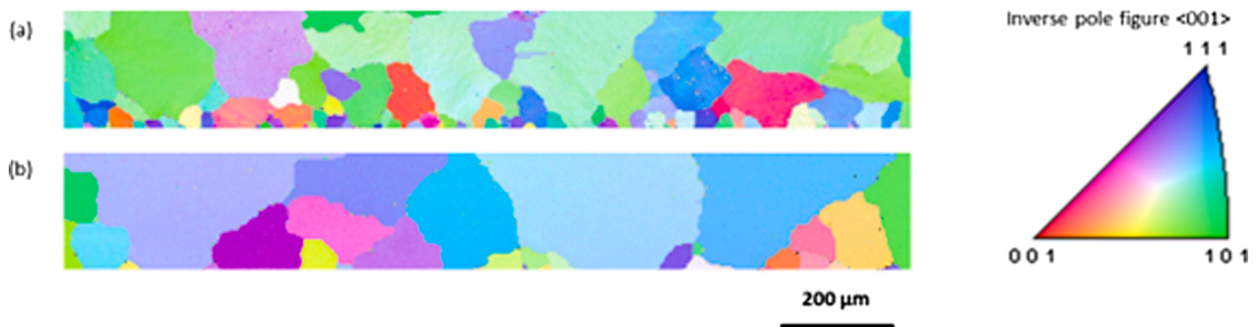
Fig. A3. EBSD inverse pole figure (IPF) maps (superimposed with grain boundary, >2^\circ ) at the edge (surface) (a) GA1 (b) GA3
