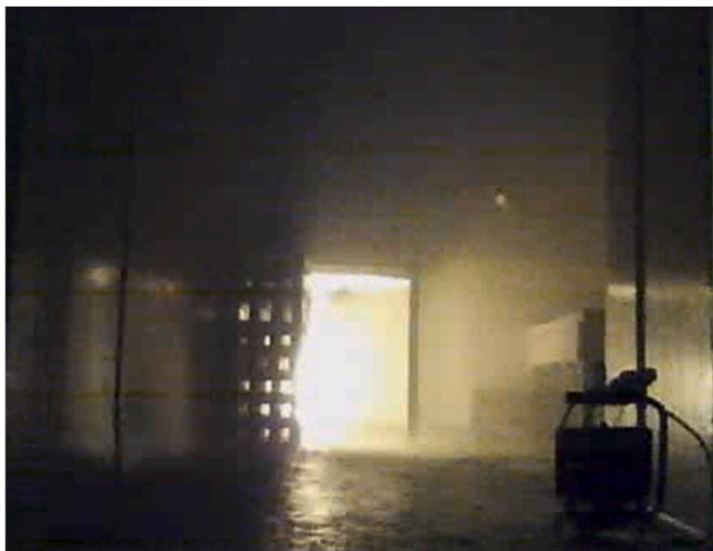
Fig. 10. The location of the fire under the table shielded the initial fire from direct water impingement. Hence, the fire was not extinguished, but controlled. Image from 08:10 (mm:ss). At this point the floor was covered by several cm of water. Photo by RISE Fire Research.
