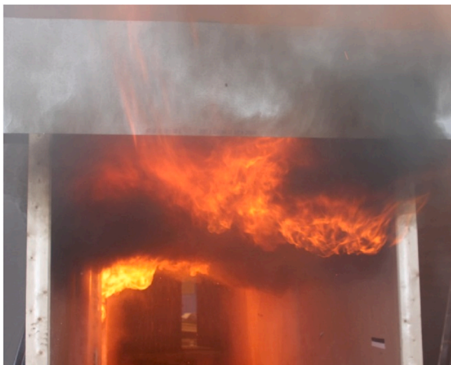
Fig. 14. Large flames quickly spread under the ceiling in the corridor. Image at approx. 6.5 min. At this point, the two sprinklers under the suspended ceiling have activated and at least one of the nozzles above the suspended ceiling. Photo by RISE Fire Research.
