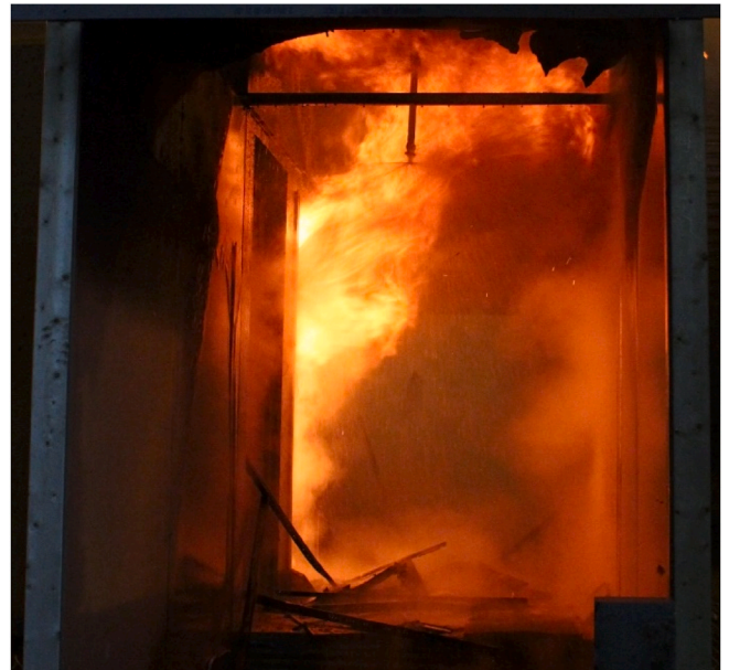
Fig. 15. Large flames emerged from the compartment into the corridor and ignited the exposed CLT ceiling and the upper parts of the walls. The suspended ceiling suffered great damage from the flames and fell down after 8.5 min, i.e., approx. 3.5 min after flames emerged into the corridor. Photo by RISE Fire Research.
