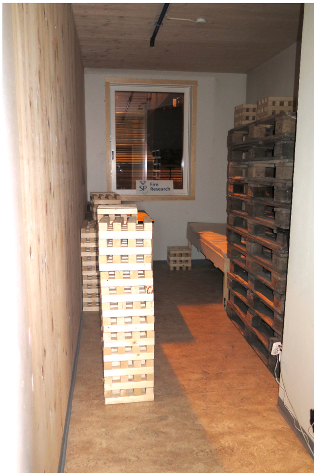
Fig. 6. Experimental setup of the compartment in Experiment 2. In the compartment, the CLT on Wall A (left) and in the ceiling were exposed. The fuel package was similar to Experiment 1 but with additional wood cribs and wood pallets (see Table 1). Photos by RISE Fire Research.
