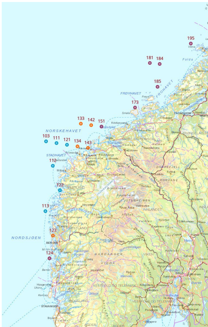
Fig. 4. Points with negative correlation close to the shore, depth \leq 200 m (color shows the monthly availability: (a) blue: \geq 6 months, (b) orange: < 6 months and \geq 4 months, (c) purple: < 4 months and \geq 1 month.)
