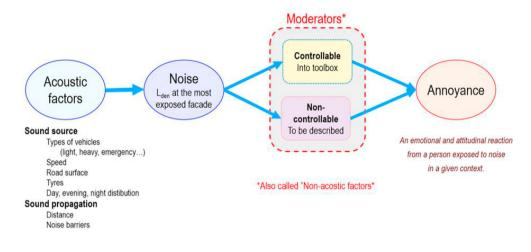
Fig. 2. Connection from acoustic factors leading to noise and moderators influencing the perceived annoyance, (FAMOS, 2022-B).
