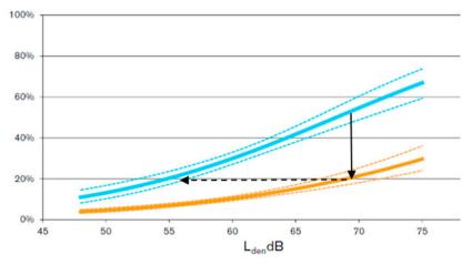
Fig. 1. The blue curve shows an example for the percentage of people being highly annoyed in a situation without moderators. The orange curve shows the percentage of highly annoyed in a situation where a moderator has been implemented.
