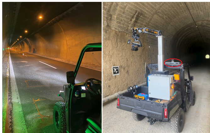
Fig. 1. Images of the autonomous cart with which we tested our localisation solution in a highway tunnel (left) and ex-train tunnel (right). Our system is mounted to the roof of the vehicle. Also visible is the crane-mounted inspection camera.
