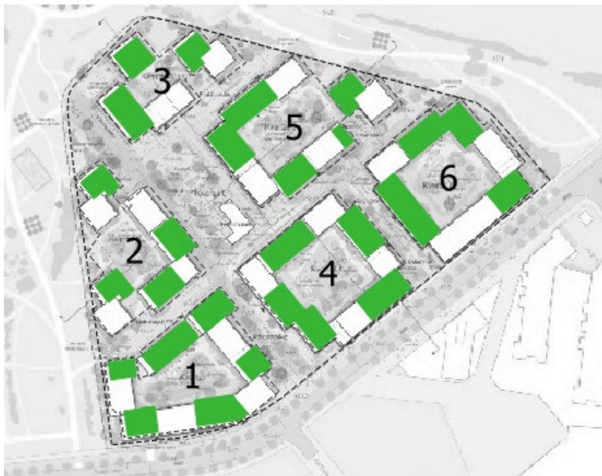
Figure 31. Map showing the roof areas for social functions and green space at Nansenløkka at the ZEN pilot area at Fornebu (48).
