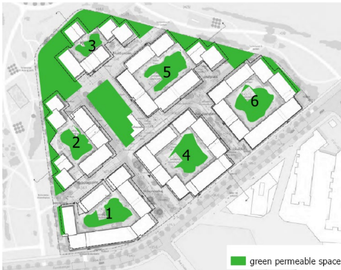
Figure 37. Green permeable area at Nansenløkka at the ZEN pilot area at Fornebu (49).
