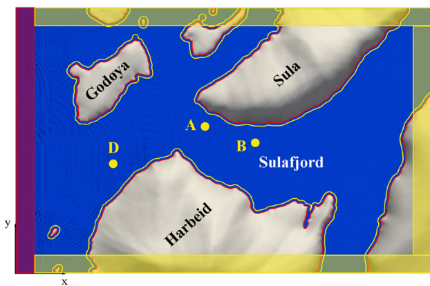
Fig. 9 Numerical configuration for the simulations of wave propagation into Sulafjord. The red box is the wave generation zone, the yellow boxes along the other three boundaries are numerical damping zone. The red lines show the coastlines and the yellow lines show the outer boundary of the coastal damping zone. The yellow dots are the wave gauges (colour figure online)
