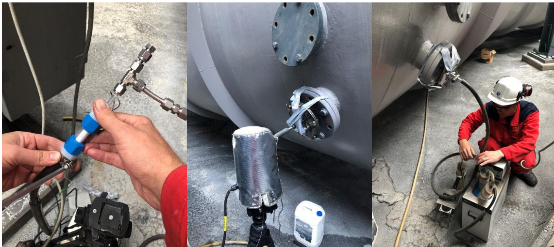
Figure 1. Sampling on SO 3 onto salt trap. The NaCl trap is shown to the left, and the connected to the sampling probe and with a heating jacket installed in the middle. To the right is shown sampling to two gas washing bottles immersed in a cryostat cooled bath with temperature of -20 °C.
