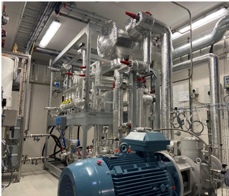
Figure 2: The ACHP prototype in the NTNU lab
