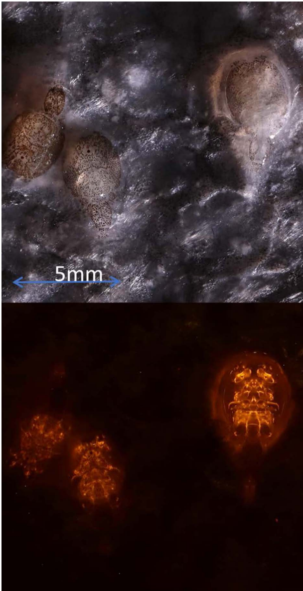
Figure 3. Three salmon lice on salmon skin. Setup described in Figure 2 were used. Top: White light source and RGB camera Bottom: 532 nm laser source, long-pass filter on RGB camera.
