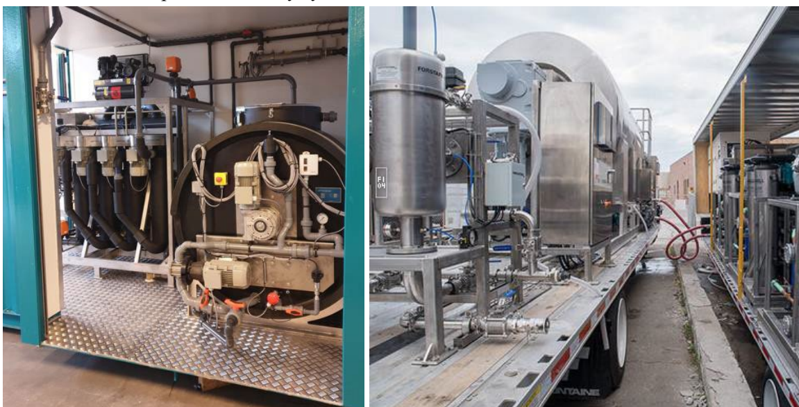
Figure 5: Left: Ice slurry system in a transportable container (Vikse, 2023). Right: Mobile unit that can deliver to different plants and harvesting sites (Deepchill, 2023).
