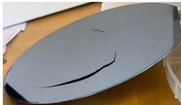
Figure 7. Onset of exfoliation of the epi-Si layer deposited on the porous Si supporting substrate using e-beam evaporation at 1000 °C.
