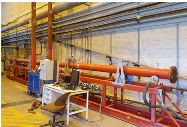
Fig. 1 Photo of the flow loop test section in horizontal position
