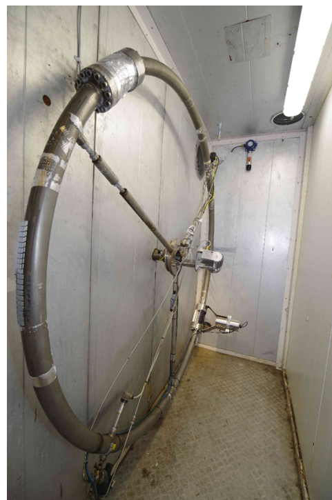
Figure 3. Wheel flow loop. The camera is the white unit sticking out from the wheel farthest away in the picture, close to the floor. It is pointing at the sapphire glass section.
