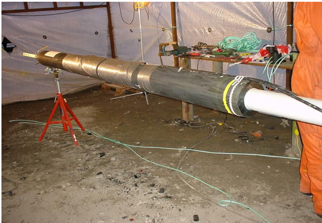
Figure A6: Thermal insulated riser.
