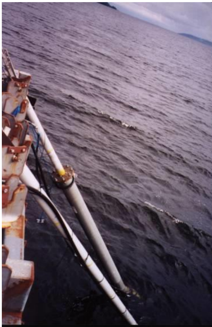
Figure A12: Pipe in pipe section mounted on the riser.
