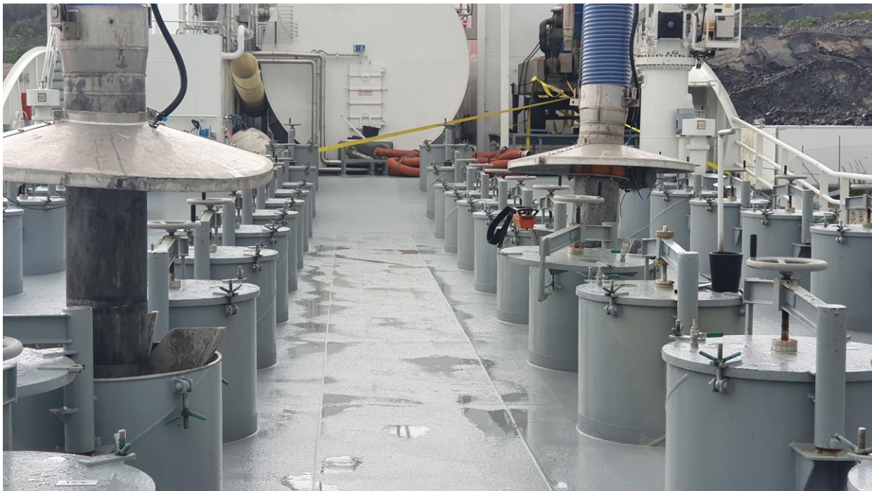
Figure 35: Land cranes lowered into silo opening. Photocells detected and loading ready to start.
