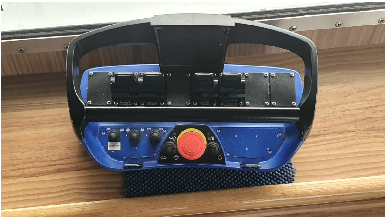
Figure 43: SSS - Remote Control Unit used for controlling the bow crane.
