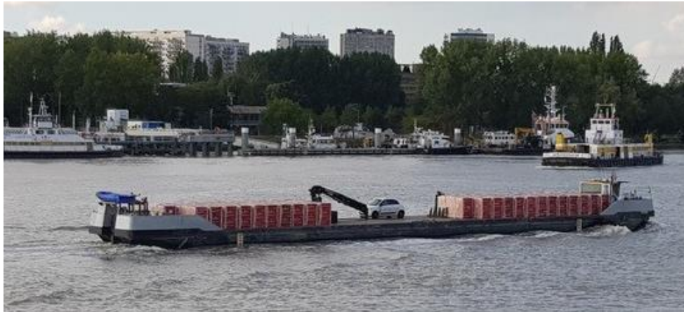
Figure 2 IWW PSB - pallet shuttle barge
