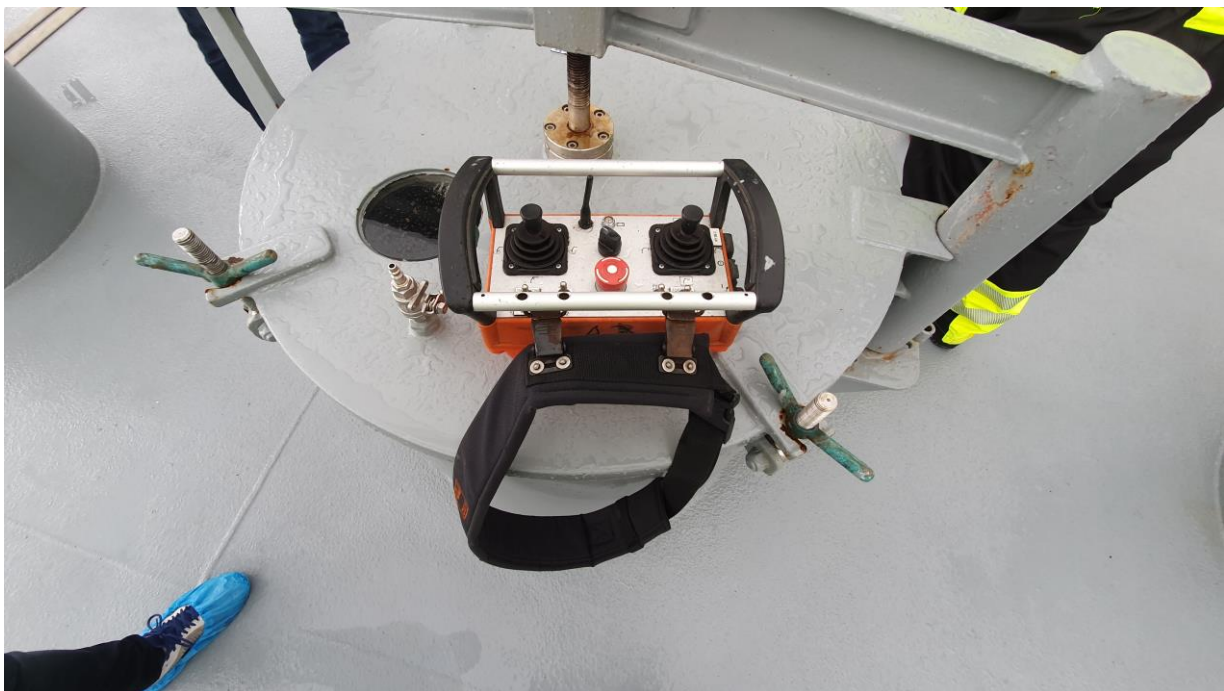
Figure 34: SSS - Remote control used to operate both land cranes.
