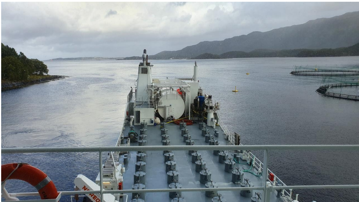
Figure 24: Deck layout of Pioner showing silo hatches distributed in four rows.
