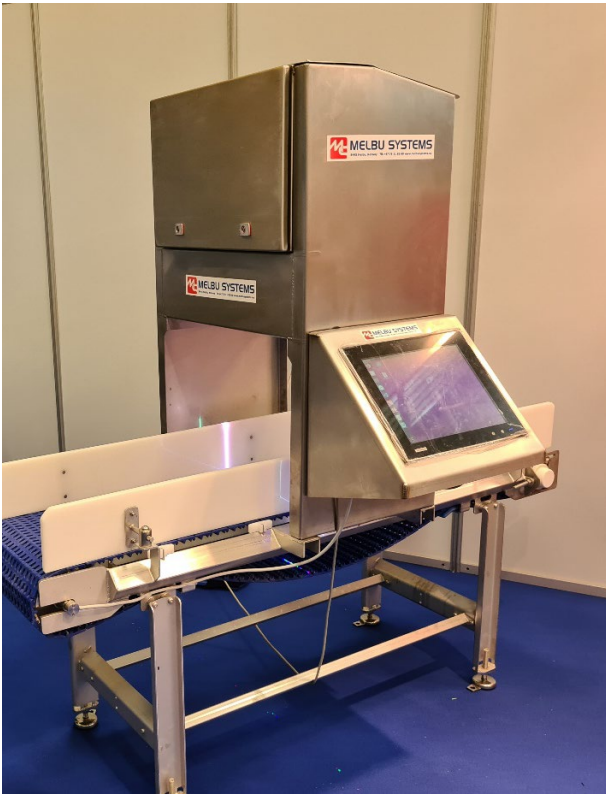
Figure 5: Assembly of CatchScanner, touchscreen and conveyor belt
