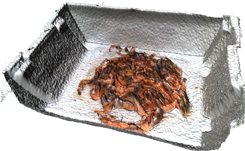
Figure 20: Colored point cloud from Azure Kinect of a batch of shrimps
