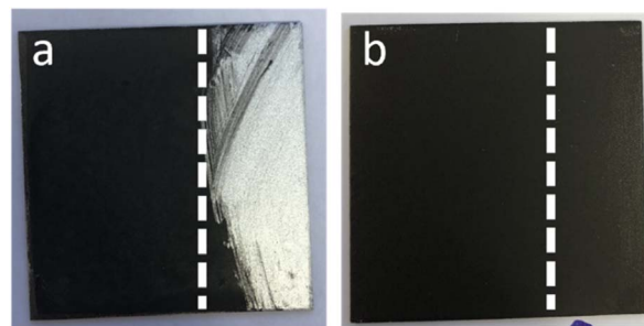
Fig. 7 Coatings on Al 2024 T-3. (a) APTES-rGO on sol-gel and (b) APTES-rGO in sol-gel. Vertical dotted lines are guides to the eye only. Wipe with moist cloth on the right side of the dotted line. Sample size = 5 \times 5 cm.
