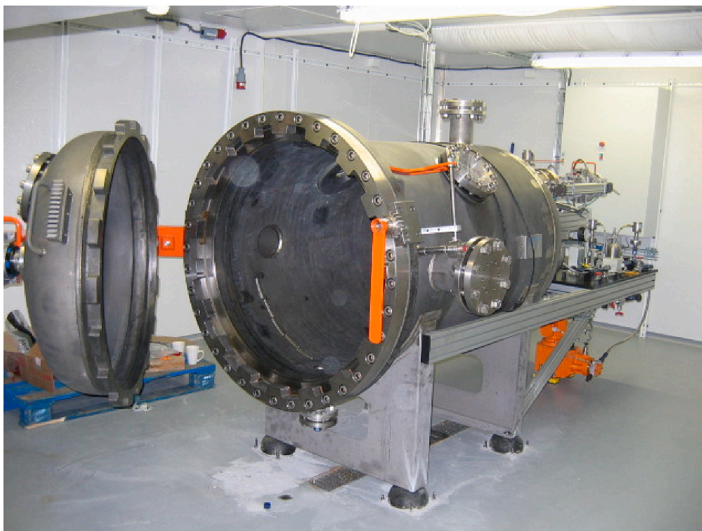
Fig. 2.1. The 1.4 m 3 Titanium pressure tank at SINTEF. Experimental conditions are found in Table 2.1.
