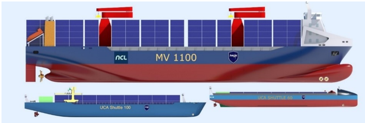
Figure 1 The AEGIS example on a mother – daughter fleet of ships, 1110 TEU mother ship in the upper part and the two daughter concepts below (60 TEU and 110 TEU)
