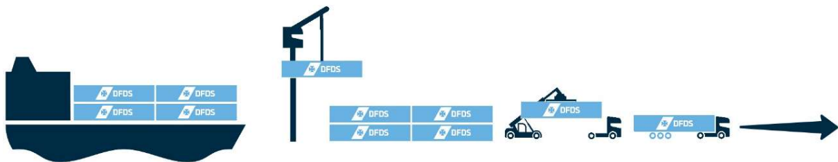
Figure 7 LoLo cargo operations (simplified).
