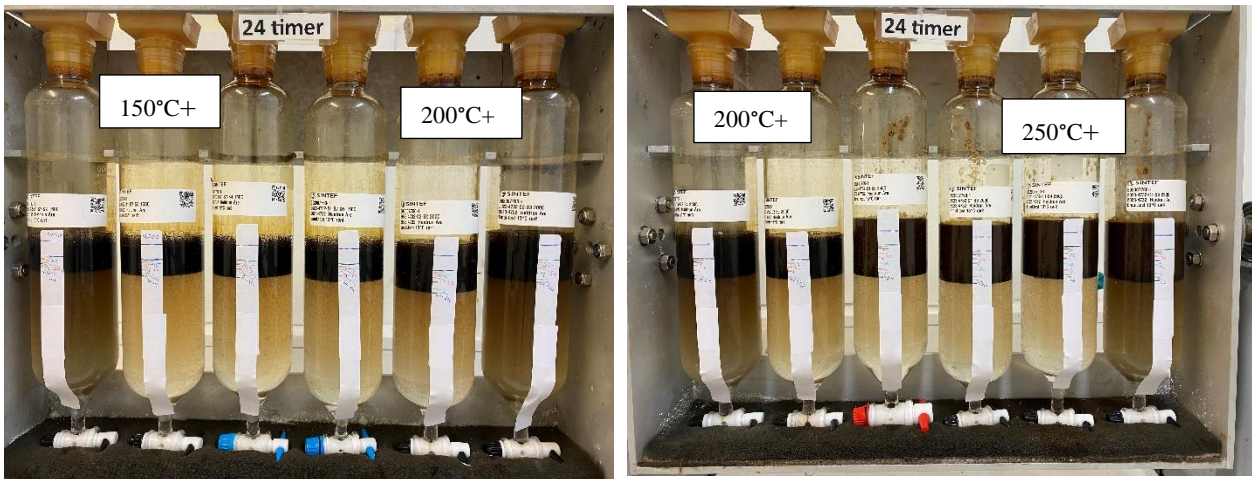
Figure 3-4 Rotating cylinders of water-in-oil (w/o) emulsions of Heidrun Åre 2023 after 24 hours at 13 °C.
