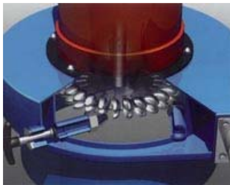
Figur 9.1. Pelton-turbin
