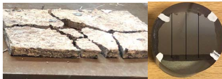
Figure 1. As-cast FSM material (left) and sample embedded in epoxy for SEM characterization (right)
