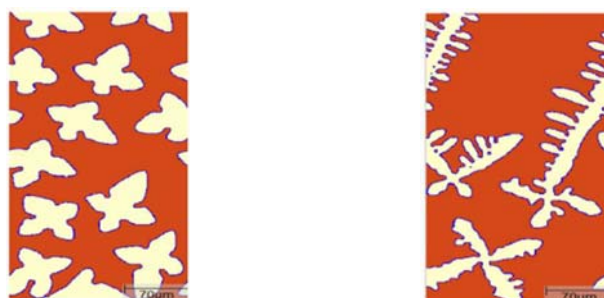
Figure 8 Nucleation and initial growth of FeSi (white) in liquid (red) at 1450K for Alloy 1 (left) and Alloy 2 (right)
