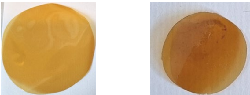
Figure 7. Images of tested membrane before (left) and after (right) the flue gas exposure for RTI case
