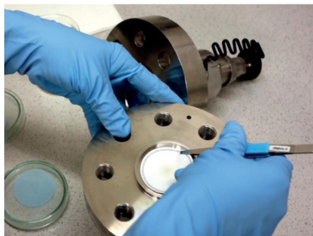
Fig. 3 – Micron filter element removal from hydrogen particle sampling adapter unit.
