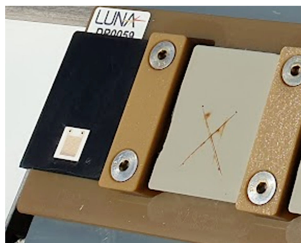
Fig. 14 The sensor package. The CorRES sensor mounted at Kjerringvik in Norwayface toward the sea (southeast) tilted 45^\circ from horizontal.
