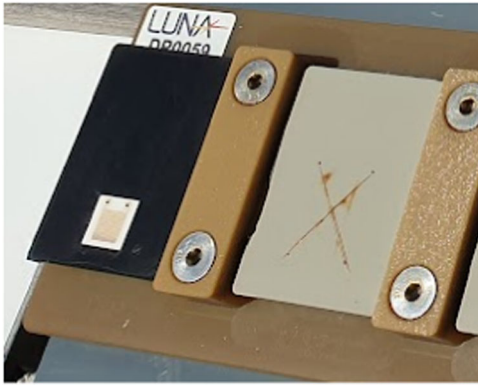
Fig. 7 The experimental setup. View of a sensor installed toward the south east sea in Kjerringvik, Norway 27 .
