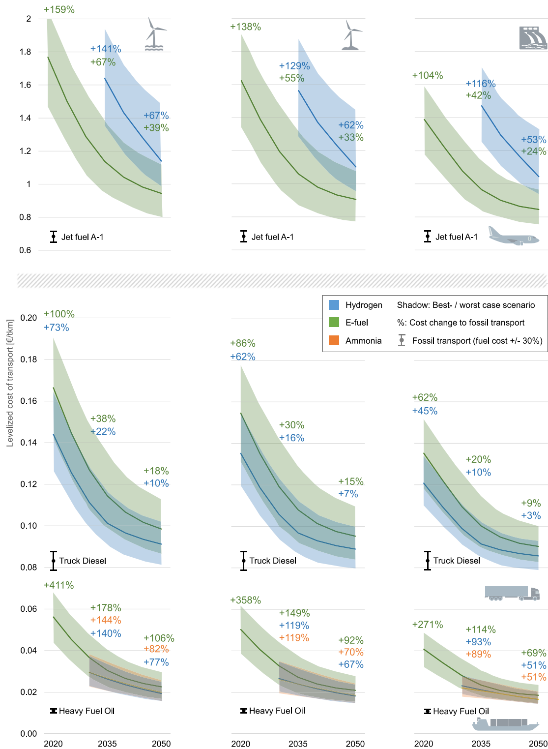
Fig. 7. Transport cost increase (percentages) in selected years driven by the fuel switch towards renewable fuels for aviation (top), trucking (center) and shipping (bottom) considering fuel options based on electricity from offshore wind (left), onshore wind (center) and hydropower (right). Shadows total the uncertainty ranges of the selected parameters.
