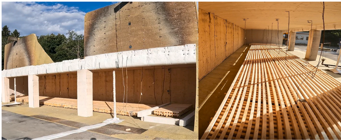
Fig. 1. Experimental setup from the outside and inside of the compartment. The small wood crib on the scale is on the right side of the left image.
