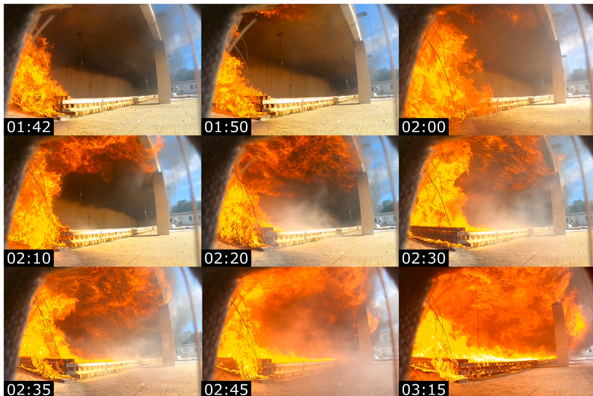
Fig. 6. Flame spread below the ceiling after ignition of CLT seen from the left side of the compartment. Time (mm:ss).
