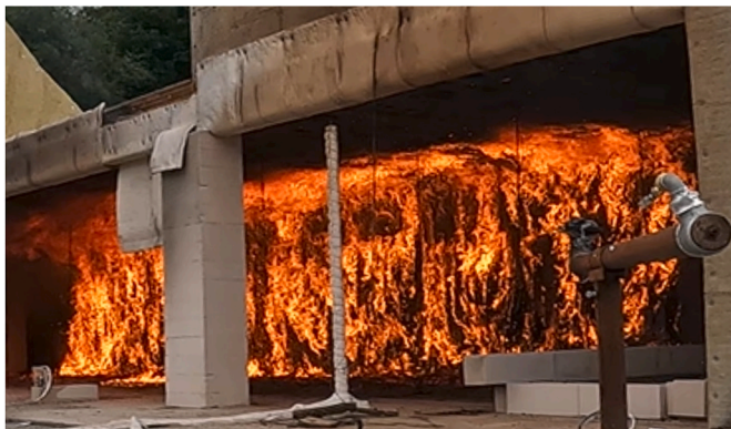
Fig. 11. In the transition to the second flashover, the full height of the back wall was burning before half of the ceiling width had been included in the fire. Photo from 74 min.
