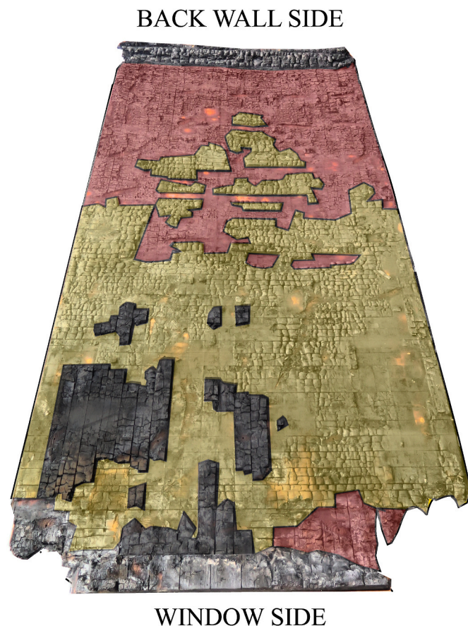
Fig. 30. Visualization of non-uniform charring for one CLT ceiling element based on a photo. Black is the 3rd layer, yellow is the 4th, and red is the 5th layer. The holes at the right and left lower corners of the window side were caused by smouldering and reignition after the end of the experiment, as this part was hard to reach with water due to safety precautions. (For interpretation of the references to colour in this figure legend, the reader is referred to the Web version of this article.)
