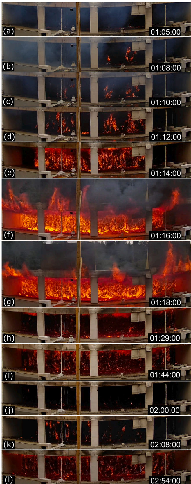
Fig. 9. (a)–(l) Development of the second flashover. (j) Fire intensity at its minimum. (k) Fire intensity at minimum compartment temperature. Time (hh:mm:ss).
