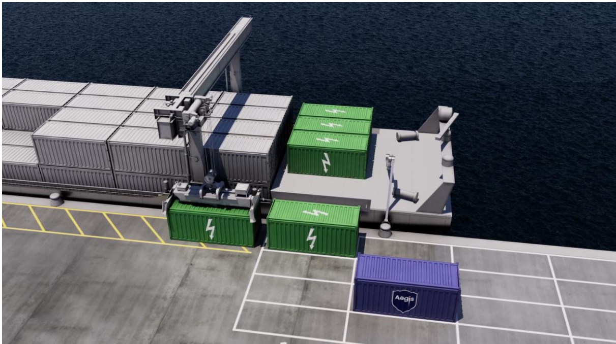
Figure 14: Battery swapping by autonomous gantry crane onboard the daughter vessel [8]
