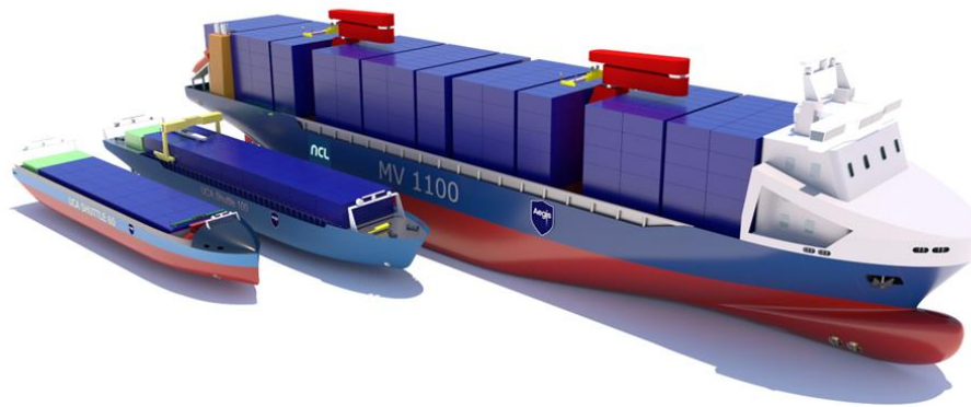
Figure 10: To the left 60 TEU daughter, middle 100- TEU daughter, to the right Mother vessel.
