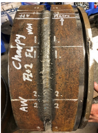
Figure 62: Clad pipe welded with Alloy 59 as filler wire at 150bar and macro close to 12o'clock position.
