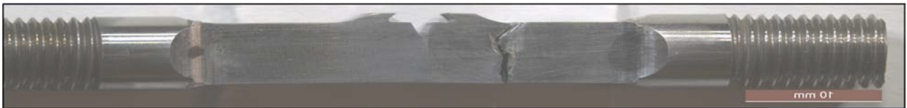
Figure 16 Picture of specimen E5-1 E1 HAZ (failure outside the notch)
