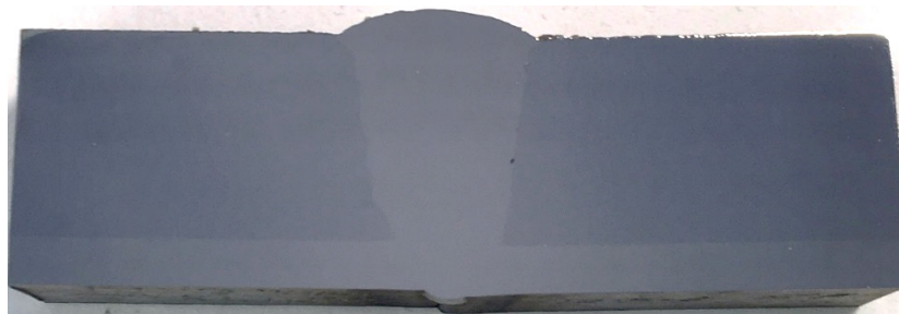
Figure 62: Clad pipe welded with Alloy 59 as filler wire at 150bar and macro close to 12o'clock position.
