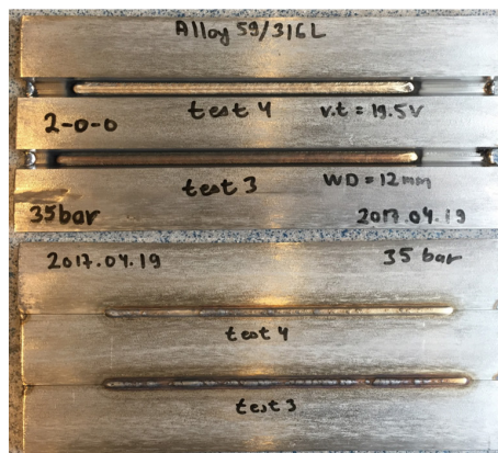
Figure 51 Over and underside of welding showing acceptable root pass penetration for the combination 316L/Alloy 59 for fit-up 2-0-0 (35bar).
