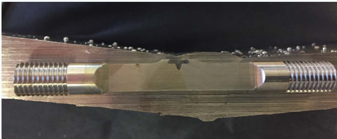
Figure 7 Picture showing that specimens are machined, so that the notch is as close external surface of the pipe as possible
