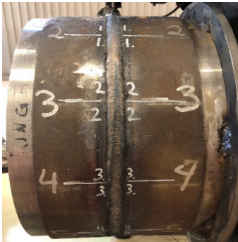
Figure 61: C-Mn (X65) welded with Coreweld HBQ as filler wire at 150bar and macro close to 12o'clock position.
