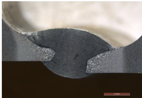
Figure 53 Root pass cross section for fit-up 2-1.5-2 using Alloy 59 as filler wires for welding C-Mn steel at 12 o'clock position (35bar).
