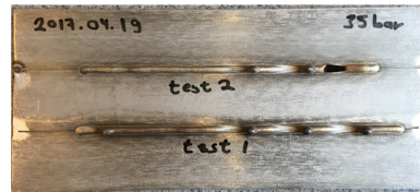
Figure 52 Over and underside of welding showing not acceptable root pass penetration for the combination 316L/Alloy 59 for fit-up 2-0-0 (35bar).
