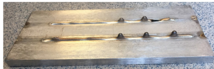
Figure 52 Over and underside of welding showing not acceptable root pass penetration for the combination 316L/Alloy 59 for fit-up 2-0-0 (35bar).
