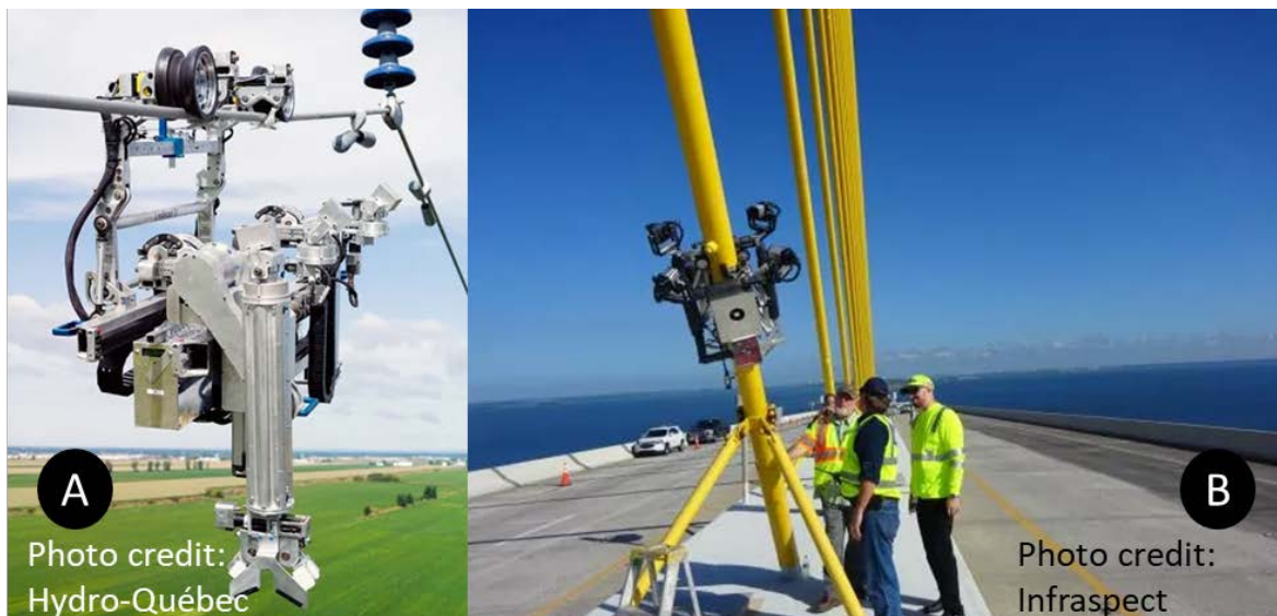
Figure 8: I&M Robots for Specific Applications. A) LineScout platform developed by Hydro-Québec that is designed for I&M of energized transmission lines, B) CableScan robotic crawler for inspection of cable-stayed bridges.
