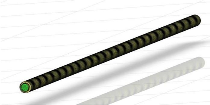
Figure 2: The meshed ADH shows the dense meshing around the perforated holes of the hose. The fan inlet at the end is shown in green.
