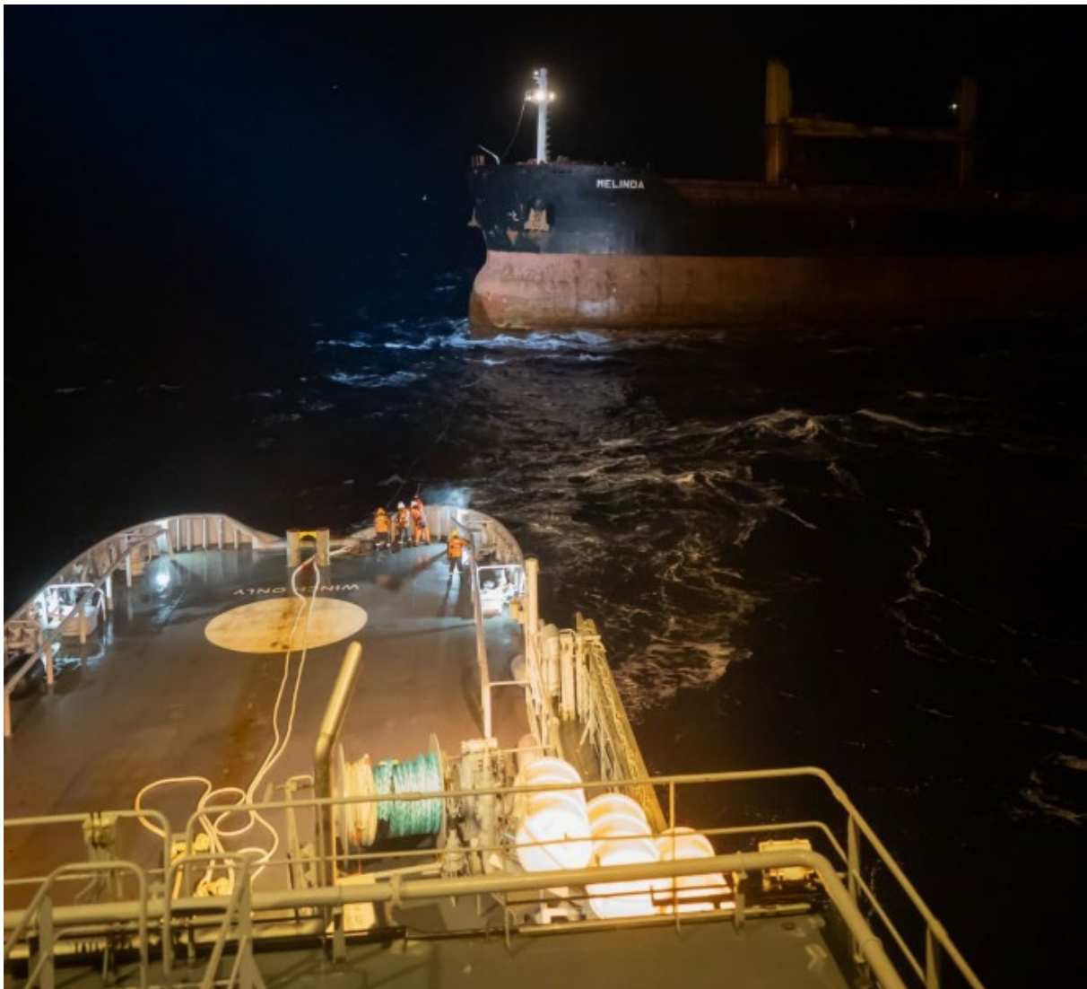
Fig. 4. Preparing the emergency towing gear on KV Harstad (Photo: Bjørn Amundsen, Norwegian Coast Guard).
