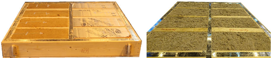
Figure 4. Left: Test specimen filled with wood fibre batt on the left half side and phenolic foam batt on the right half side. Right: Test specimen filled with wood fibre loose-fill insulation (manually packed) between the Hunton I-joists (left) and Masonite I-joists (right). The fibreboard is not installed.
