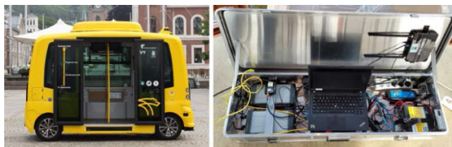
FIGURE 4. The bus from EasyMile (left picture) was used for the practical test in Drammen. The box on the right shows the installation of the receivers and the computer/modem used for remote access and to receive GNSS corrections for all receivers.
