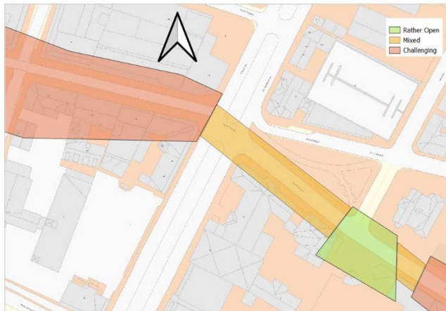
FIGURE 5. Example of the three surrounding types used to distinguish between GNSS conditions on the test site.
