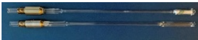
Figure 4. Upper: Standard reactor with sample, quartz and locking-pin. Lower: Empty large reactor.
