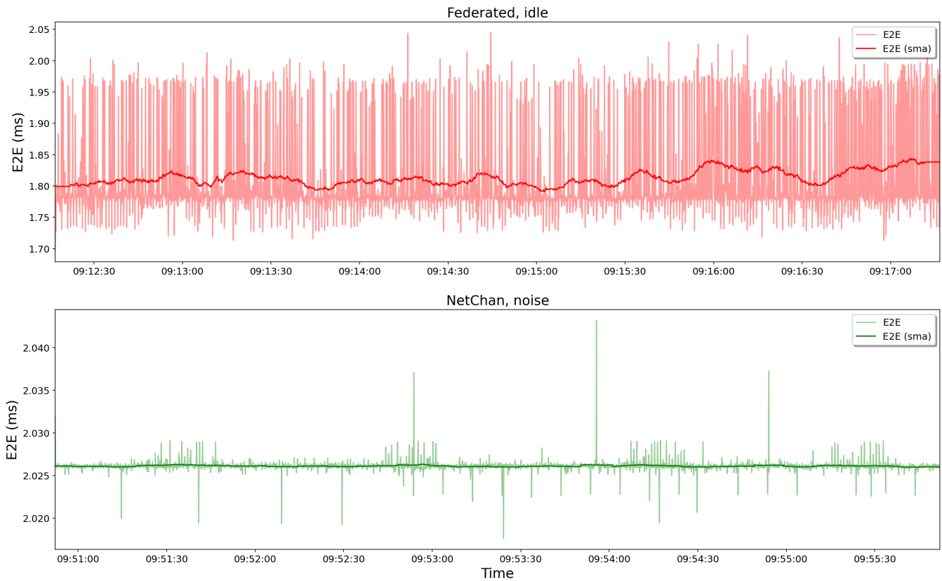
Figure 5: E2E comparison of an idle, federated system and LF using net_chan under severe network load. Same dataset as used to generate Table 2
