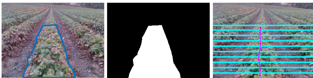
Figure 10. Ground Truth Centerline by manual annotation. The left image is the raw RGB image from the camera. The middle image is the binary mask generated by freehand masking; the final image corresponds to the centerline of the crop row as ground truth (pink).
