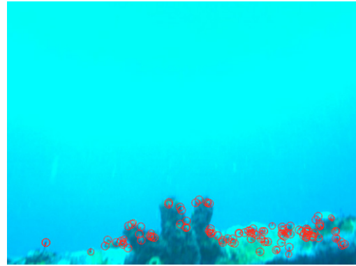
Fig. 3. Image acquired by an Aqua2 AUV during navigation over the Stavronikita shipwreck in Barbados. Features are detected only at the lower part of the image.
