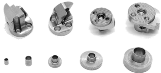
Fig. 4: Examples of shiny parts relevant for pick-and-place operations in Use Case 2. Top row: cutting heads. Bottom row: nozzles.
