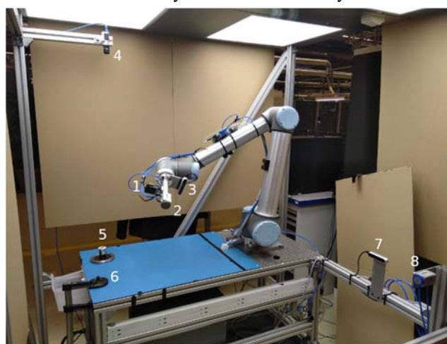
Fig. 7. Setup for Use Case 2. Components include (1) a two-finger gripper for handling nozzles, (2) a magnetic gripper for handling cutting heads, (3) a RealSense 415 camera – all three mounted on a UR10 robot manipulator from Universal Robots, (4) a Basler monochrome camera for precision estimation of 2D position and orientation of a cutting head held by the robot's magnetic gripper, (5) a jig to fix the cutting head's position and orientation for parts assembly, (6) a pallet for nozzles, and a reorientation station for cutting heads. The reorientation station is composed of (7) a Realsense 415, and (8) a magnetic gripper. All grippers are actuated by pneumatics.
