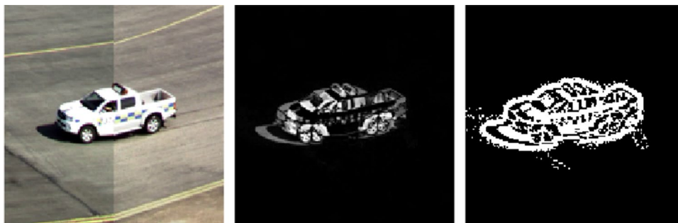
Fig. 5 In a given image region (left), changes are detected by taking the absolute difference of consecutive frames (middle) and thresholding (right). This figure is not included in the article’s Creative Commons licence
