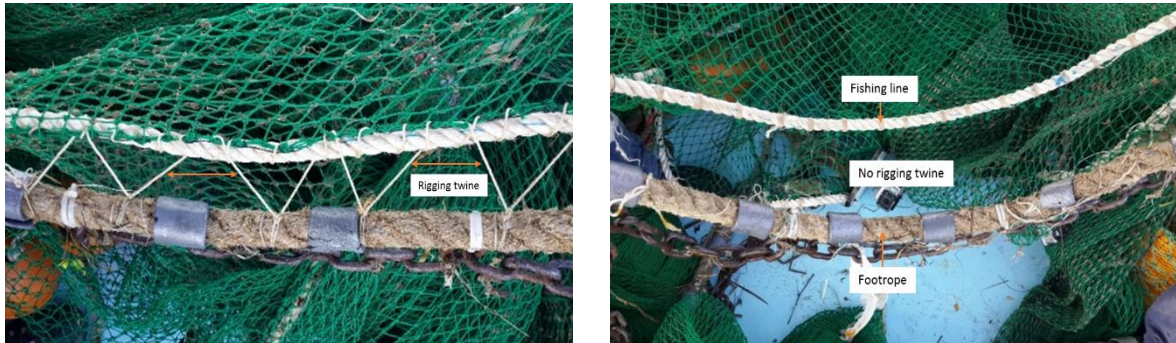
Fig. 2. Standard ground gear (left), modified ground gear (right)
