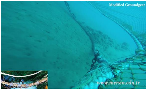
538 Fig. 3. Sequence taken from footrope camera showing that the central gap we created between footrope and fishing line before 539 settlement (a) and posture of the modified ground gear on the seabed after settlement (b) in two consecutive frames.
