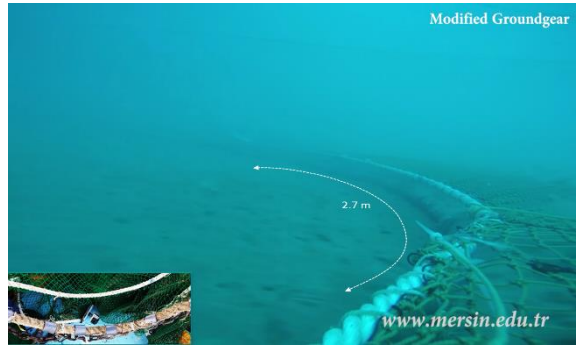
538 Fig. 3. Sequence taken from footrope camera showing that the central gap we created between footrope and fishing line before 539 settlement (a) and posture of the modified ground gear on the seabed after settlement (b) in two consecutive frames.
