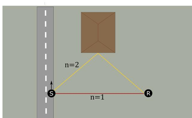
Figure 2: The paths  $n$  from a source  $S$  to a receiver  $R$  seen from above when a reflecting building induces an additional path  $n = 2$ . There will also be paths in the vertical plane, which are not shown in the figure.
