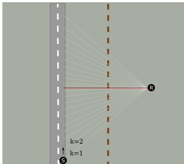
Figure 1: The figure illustrates a road-traffic source  $S$  in position  $k$ . The sound rays that reach the receiver  $R$  when seen from above is illustrated in gray. The red line illustrates the position and ray path that will give the maximum level in this specific symmetrical case. The brown stippled line is an infinitely long noise barrier parallel to the road.
