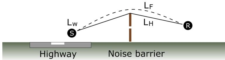
Figure 3: Illustrates the setup for the computational example for road traffic noise. The source is denoted  $S$  and the receiver  $R$ . Both paths for favourable and homogeneous atmosphere is illustrated, but only favourable atmosphere has been used in the example.
