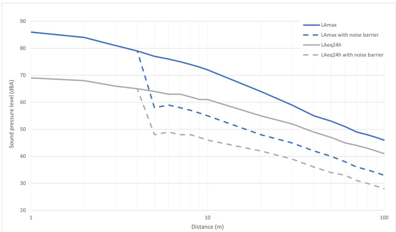
Figure 4: Source height: 0.05 m, Receiver height 1.5 m, Ground condition: soft surface. In this example a 2 m high noise barrier has been placed 4.5 meter from the roadside. The speed of the vehicle is set to 50 km/t with AADT 4000. The car's sound power level is set to 100 dB and its frequency spectrum has been taken from HB 47 [11].
