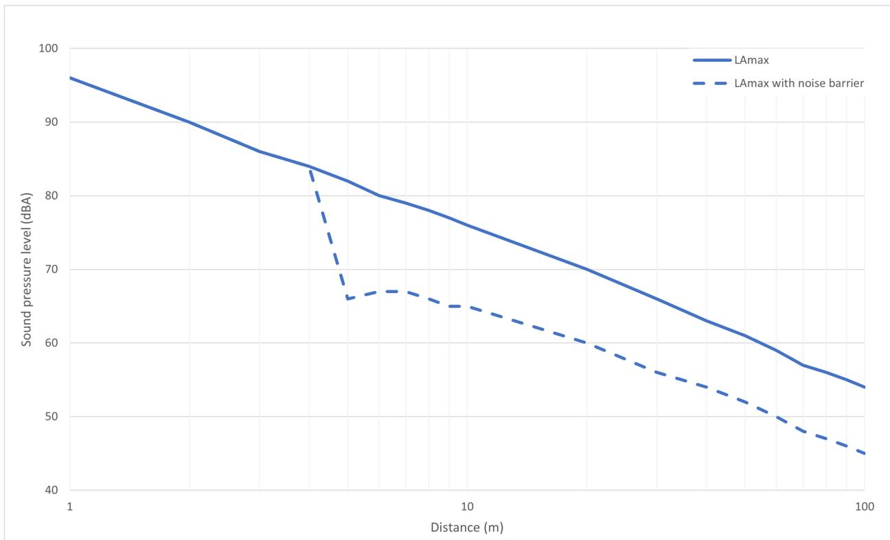
Figure 7: Calculation results from industry source. Source height: 1.5 m, receiver height 1,5 m, ground conditions soft surface. Sound power level 100 dB with flat spectrum.
