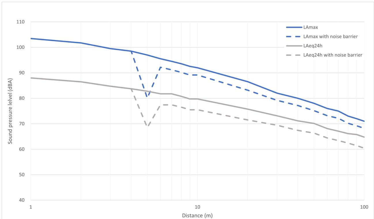
Figure 6: The 10 first meters is simulated to be a locomotive. The source height is 0.5 m, and the receiver height is 4 m. Ground condition soft surface has been used. In this example, a 2 m high noise barrier placed 4.5 meters from the roadside has been implemented. The train speed is set to 120 km/h, and 4000 passes in 24 hours has been used. The train Sound power level is set to 100 dB, and the frequency spectrum was found in HB 47 [11]
