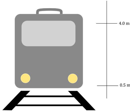
Figure 5: Illustrates the two source positions for a railway source in Cnossos-EU.
