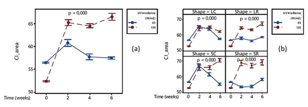
Figure 8. Effect of UV irradiance intensity and shape on the carbonyl index of PET.
