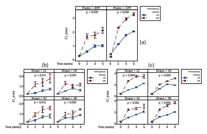
**Figure 6.** Summary of carbonyl index results for CPP and BPP. (**a**) Carbonyl index over time per plastic. (**b**) Carbonyl index over time for BPP per shape. (**c**) Carbonyl index over time for CPP per shape.
