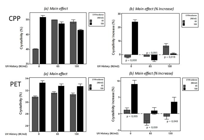
**Figure 11.** Percentage crystallinity of the BPP, CPP, and PET materials generated in the pretreatment dry UV exposures following subsequent UV exposure under aqueous (seawater) conditions. The percentage change in crystallinities relative to the values calculated for the pretreatment study are also presented for BPP (b), CPP (b), and PET (b).
