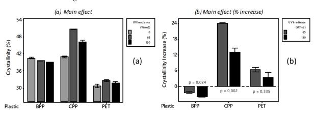
**Figure 3.** (a) Degree of crystallinity for the BPP, CPP, and PET under 65 W/m<sup>2</sup> and 130 W/m<sup>2</sup> UV irradiances, and (b) percentage change in crystallinity after 6 weeks of exposure to UV.
