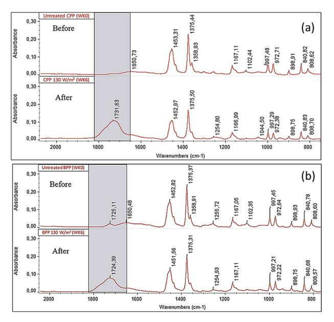
**Figure 7.** FTIR spectra of (**a**) CPP and (**b**) BPP showing the development of the carbonyl peak in both materials following six weeks of exposure to UV irradiance at an intensity of  $130 \text{ W/m}^2$ .
