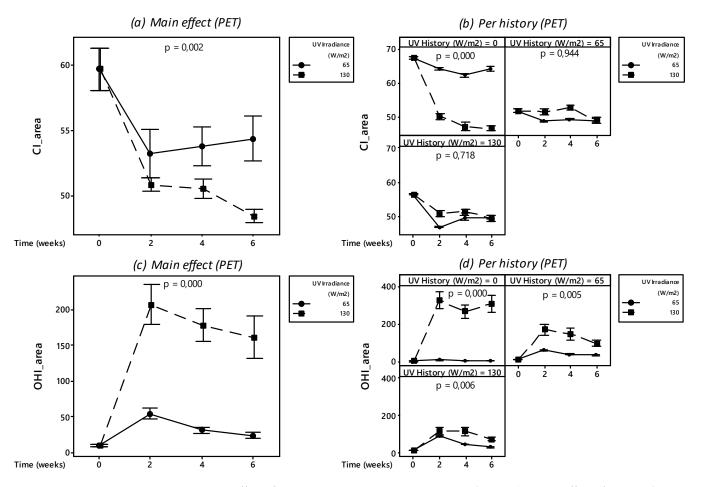
**Figure 13.** Effect of UV intensity on PET in seawater conditions: (a) Main effect of UV irradiance on CI over time (weeks) for PET; (b) CI over time (weeks) for PET with different UV histories; (c) main effect of UV irradiance on OHI over time (weeks) for PET; (d) OHI over time (weeks) for PET with different UV histories.
