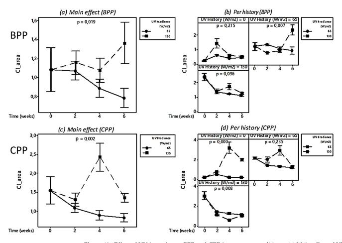
**Figure 12.** Effect of UV intensity on BPP and CPP in seawater conditions: (a) Main effect of UV irradiance on CI over time (weeks) for BPP; (b) CI over time (weeks) for BPP with different UV histories; (c) main effect of UV irradiance on CI over time (weeks) for CPP; (d) CI over time (weeks) for CPP with different UV histories.
