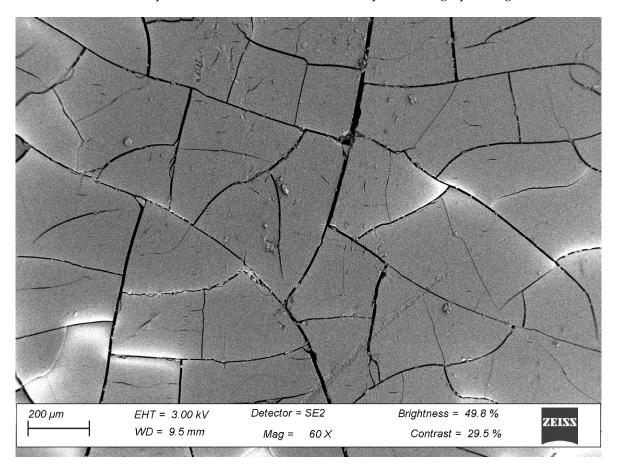
Figure 4. SEM image of UV-treated PP at 130 W/m<sup>2</sup>.
