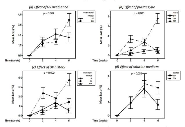
**Figure 10.** Effect of (a) UV irradiance  $(W/m^2)$ , (b) plastic type, (c) UV history  $(W/m^2)$ , and (d) solution medium on mass loss (%) over time (weeks) for the UV beaker tests.
