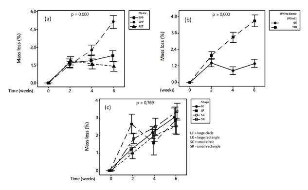
**Figure 2.** Main effects of (**a**) plastic type, (**b**) UV irradiance intensity, and (**c**) plastic shape and size on mass loss over time (up to 6 weeks) for the UV exposure studies.
