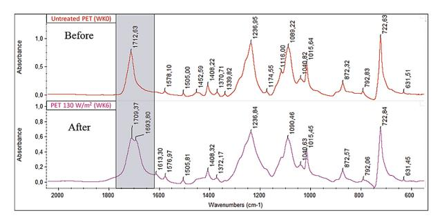
**Figure 9.** FTIR spectra of PET indicating the broadening of the carbonyl peak and formation of acids following six weeks of exposure at a UV irradiance of  $130 \text{ W/m}^2$ .
