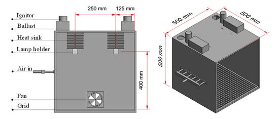
Figure 1. Schematic of the UV chamber used in this investigation.
