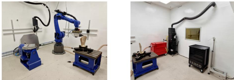
Figure 3: Finished layout inside the cell. The left image shows robot and tilt/rotation table, note build head hanging on tool-changer on the wall. The image to the right shows the Ruwac high-vacuum exhaust system, note ventilation slits close to the ceiling.
