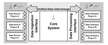
Fig. 1. Conceptual architecture for data analytics on an Android gateway.
