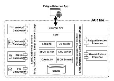
Fig. 2. AnTS framework for fatigue detection using fitness trackers.
