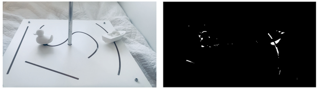
Figure 10. DMD results on foreground object with same pixel intensity as background object. The original frame is displayed to the left and the filtered foreground is displayed to the right.
