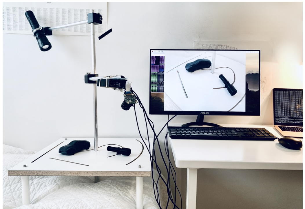
Figure 3. The Raspberry Pi 4B and Raspberry Pi camera mounted on the camera tripod.
